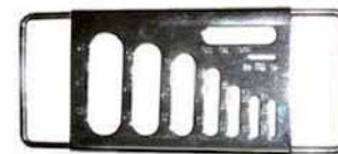
Figure 9: The Flakiness Index test gauge and Flakiness Index slotted sieves
