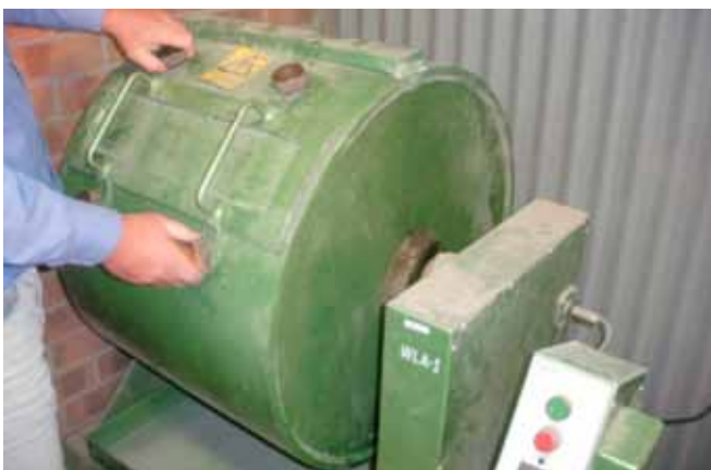
Figure 11: LA machine and test sample
