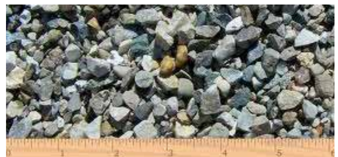
Figure 13: Examples of river gravel with crushed and uncrushed face
