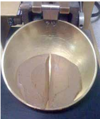
Figure 14: Liquid limit device with sample
