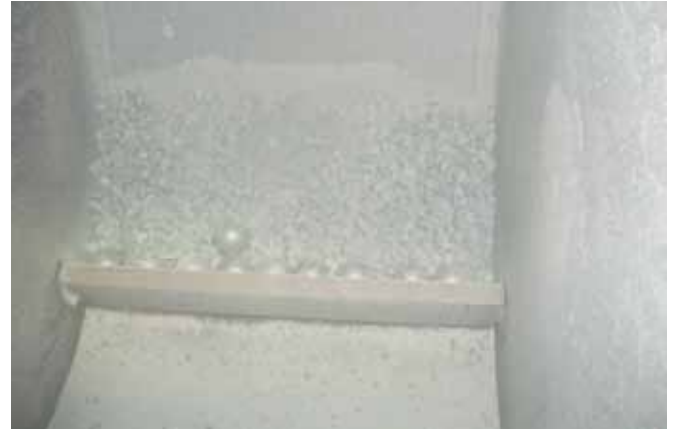
Figure 12: LA machine test sample
