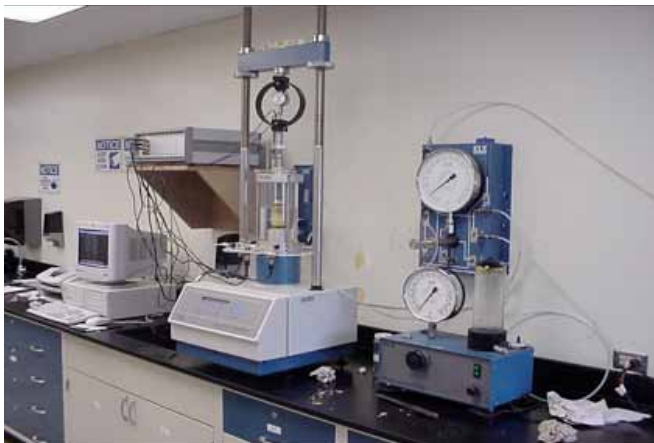
Figure 18: A view of typical Texas Triaxial testing equipment
