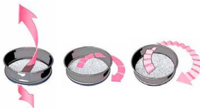
Figure 6: Shows the actions required when proof sieving to obtain the desired outcome when proof sieving
